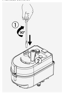
In the case of power failure or for service purposes, user can manually operate with the actuator:
